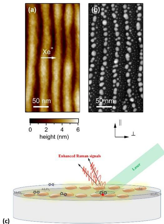
Fig.1 : (a) AFM image of an  $\text{Al}_2\text{O}_3$  thin film etched with 1 keV- $\text{Xe}^+$  ions. (b) HAADF-STEM plan view image of  $\text{Al}_2\text{O}_3$ -capped Ag nanoparticles grown on a rippled  $\text{Al}_2\text{O}_3$  thin film. (c) Sketch of the SERS substrate.
