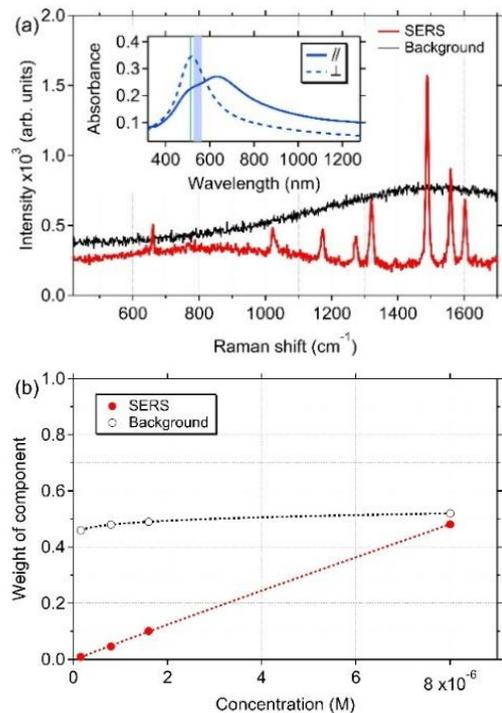
Fig.2 : a) Multivariate analysis of 108 SERS spectra recorded from an  $\text{Al}_2\text{O}_3/\text{Ag}/\text{Al}_2\text{O}_3$  SERS substrate (5 nm thick capping-layer) at a laser excitation wavelength of 514.53 nm with transverse polarization of the excitation. Inset: Optical absorbance spectra of the trilayer with transverse or longitudinal polarization. (b) Respective weight of the 'background' and 'SERS' spectral components as a function of the bipyridine concentration.
